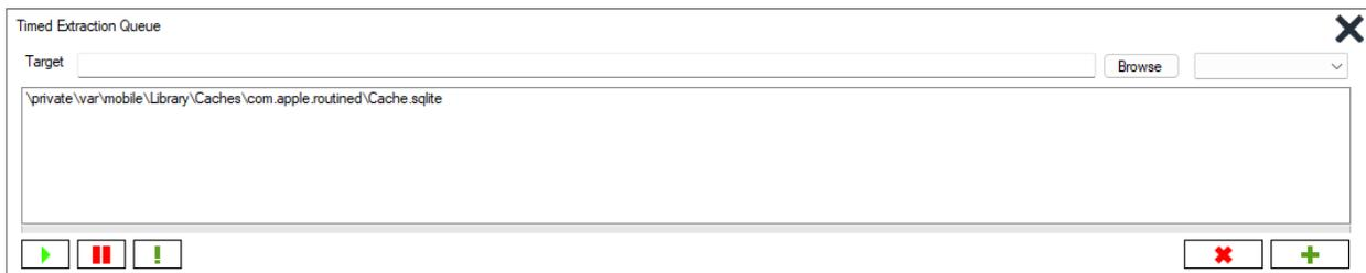
Use the Target field to select a folder to extract the files to and use the drop down menu to select the extraction frequency.
