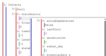
**Embed UID Data** - Will build the tree and substitute the UID value for the data it represents. Here, we see the same data as above, except instead of showing a UID Value of 5, the actual value of Node 5 is shown in its place.
